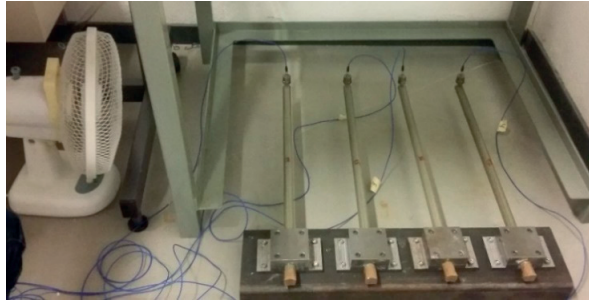
Figure 5.12 Setup of EMM-ARM
