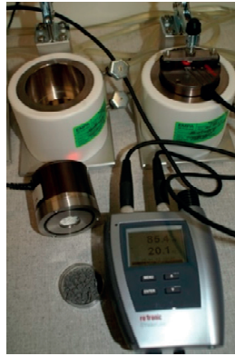
Figure 3.10 Setup for internal relative humidity measurement
