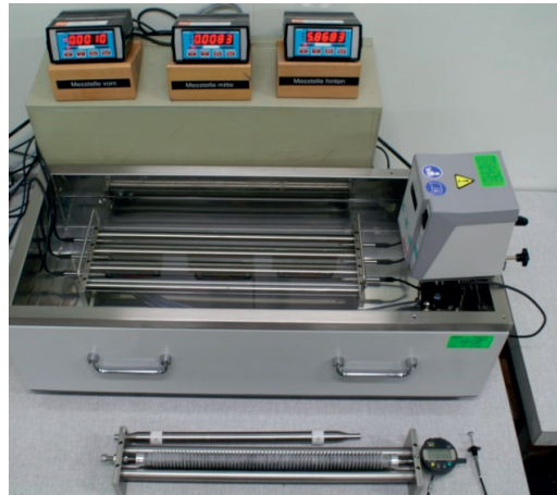
Figure 3.9 Setup for autogenous shrinkage measurement
