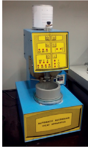
Figure 3.8 Setup for Vicat needle test
