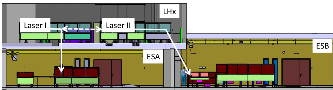
Figure 10. Laser I and Laser II are located in the laser lab LHx, on the floor above the two experimental stations Alvra (ESA) and Bernina (ESB).
