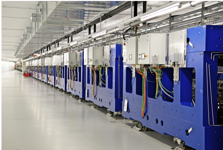
Figure 3. SwissFEL Aramis undulator line with a total length of 60 m (4 m each module and 0.75 m intersection).
