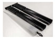
Fig. 3. Silicone based compliant arm and mold.
