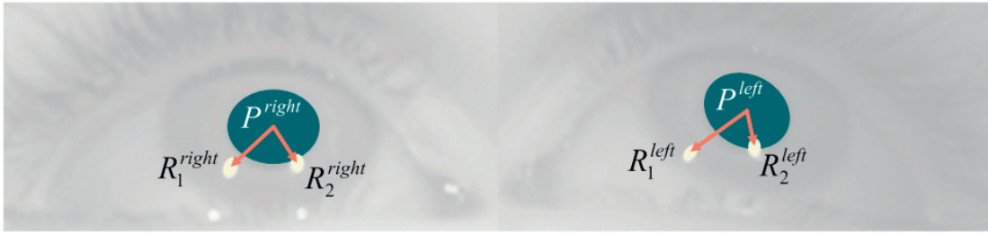
Figure 2.7 – Pupil-glint vectors that are fed into the mapping function to estimate the gaze. Image taken from [Sesma-sanchez et al., 2012].
