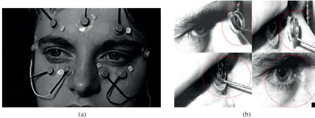
Figure 2.2 – Intrusive eye tracking techniques based on: (a) electro-oculography , (b) contact lens (search coil) method [Duchowski, 2000].
