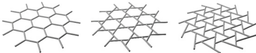
Figure 2. Examples of RF grid configurations studied by Parigi and Kirkegaard [5].
