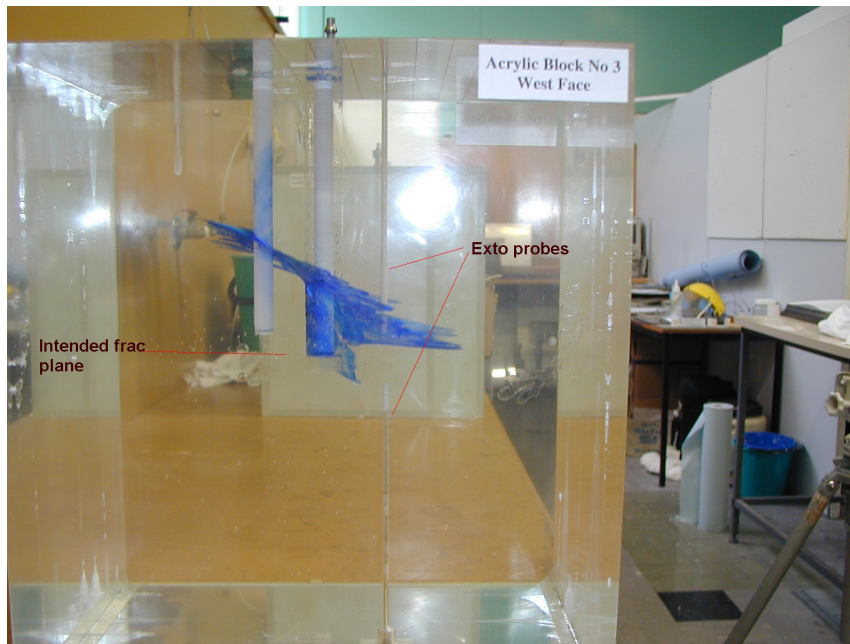
Figure 6. Complex HF geometry in the near-wellbore region exhibiting completion interface debonding (micro-annulus), re-orientation toward the far-field preferred fracture plane with fracture front segmentation due to mixed mode fracturing (Photo courtesy of Rob Jeffrey & Jean Desroches). Experiments performed in PMMA with a Newtonian fracturing fluid.
