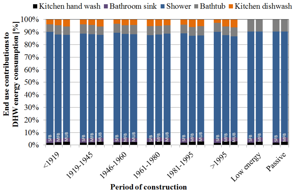
Figure 2.8: End-use contribution to household DHW energy demand (SFB - single family building, MFB - multifamily building, MUB: mixed-use building)
