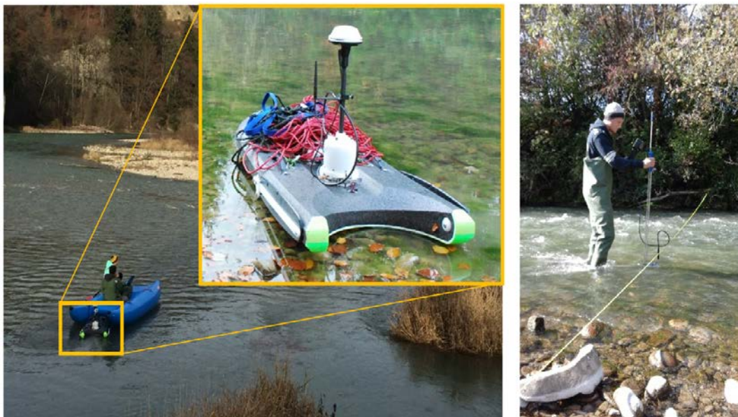
Figure 3: Tools used to measure flow velocity: on the left side SonTek RIVERSURVEYOR®, and on the right side the SonTek FLOWTRACKER®. Images were taken in the Sarine River, Switzerland.
