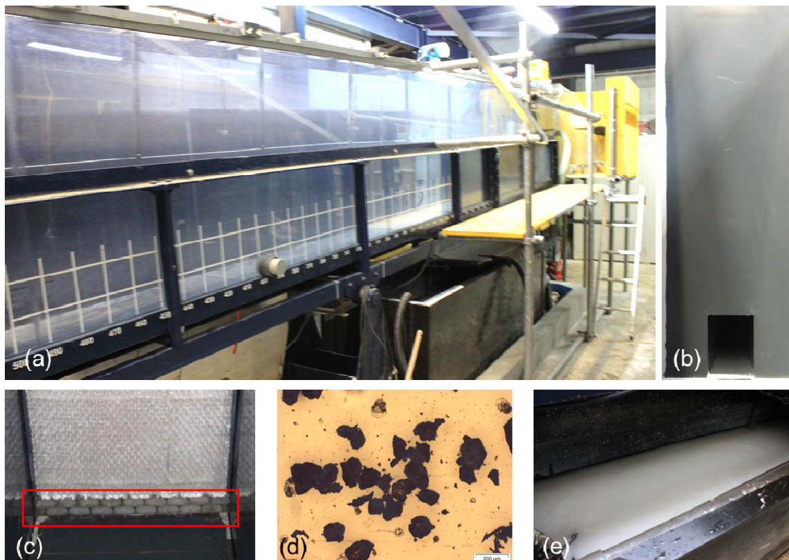
Figure 1. Experimental set-up showing (a) the main flume (b) the bottom outlet and the wall (c) the inlet highlighted in red below part of the diffuser (d) a microscopic photo of the sediment material and (e) the sediment-water mixture in the mixing tank before the beginning of a test.
