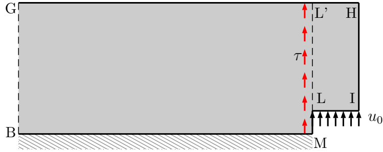
Figure 10: Resultant force scheme for initial loading due to the imposed displacement u_0 .
