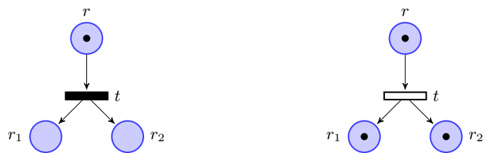
(a) Initial marking for the request \{r\} (b) Final marking for the request \{r\}
