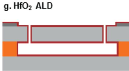
Figure 4.9 – Schematic of the added fabrication step used to partially filled the resonator gaps with HfO 2 .
