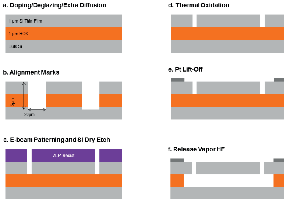
Figure 4.1 – Schematic of the fabrication process used to create air-gap MEMS resonators.
