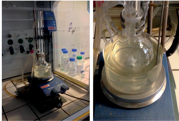
Figure B.1 – PVDF-TrFE preparation setup: (left) complete setup (magnetic stirrer, round-bottom flask, oil bath, condenser and thermometer) and (right) details of the PVDF-TrFE power and the magnetic stir bar.
