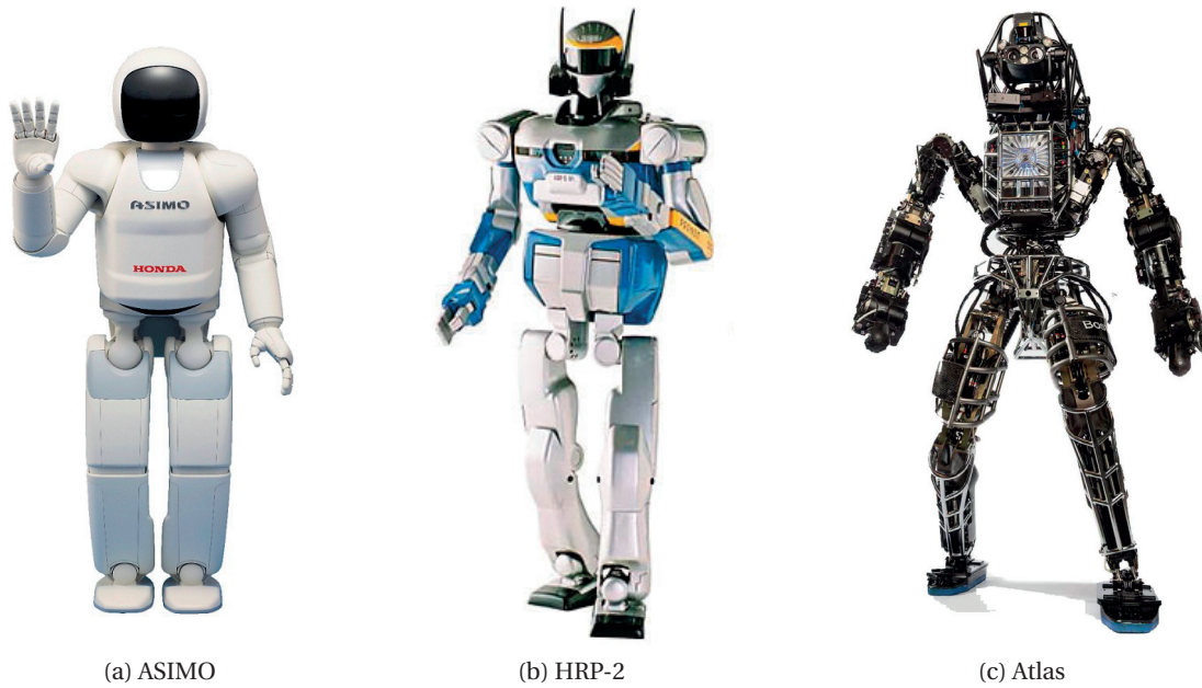
Figure 1.1: Humanoid robots achieving dynamic walking: (a) ASIMO developed by Honda (image taken from http://asimo.honda.com/ ); (b) the HRP-2 platform developed by the Intelligent Systems Research Institute (AIST, Japan) (image taken from http://www.plasticpals.com ); (c) the Atlas robot developed by the American robotics company Boston Dynamics (image taken from http://www.bostondynamics.com/robot_Atlas.html ).
