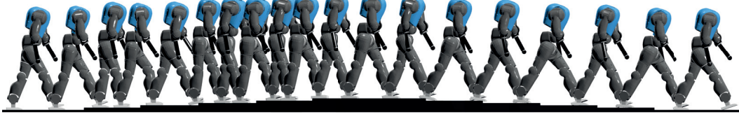
Figure 9.14: Snapshots from Experiment 7: COMAN walked blindly on an ascending and descending stair. Step length was automatically adapted to the environment, without changing the controller. At the end of the stair, COMAN retrieved its initial gait, thanks to the CPG.
