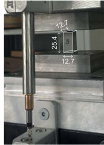
Figure 3.4: Compressive experimental set-up (dimensions in mm)
