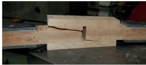
Figure E.3: Typical failure of the double-lap timber joint
