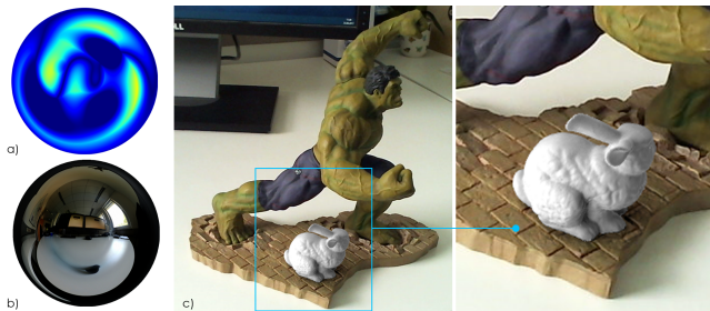
Figure 9: Augmented Reality rendering using our light estimation and the real world object as light probe. (a) Visualization of the difference between our estimated lighting and (b) the current real world lighting, which has been directly captured using a 360 camera. (c) Augmentation of a virtual bunny using the estimated lighting.
