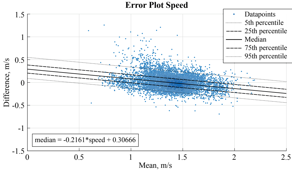
Figure 12.6 – Error plot for the instantaneous speed estimate. The correlation adjusted 5 th , 25 th , median, 75 th and 95 th percentiles are -0.21, -0.10, -0.01, 0.08, and 0.25m/s, respectively.
