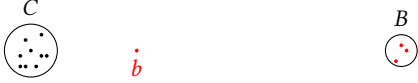
Figure 2: Selecting the vector that minimizes the sum of the squared distances to other vectors does not prevent arbitrary vectors proposed by Byzantine workers from being selected if f \geq 2 . If the gradients computed by the correct workers lie in area C, the Byzantine workers can collude to propose up to f - 1 vectors in an arbitrarily remote area B, thus allowing another Byzantine vector b , close to the barycenter of proposed vectors, to be selected.
