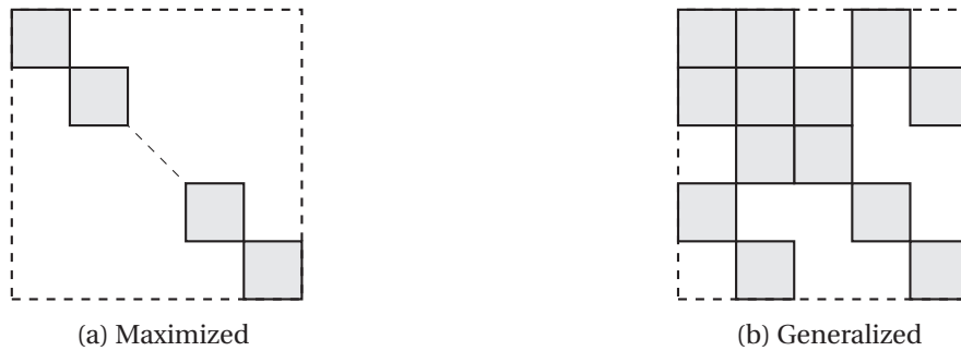
Figure 2.3 – Structural differences in inertia matrices between maximized and generalized RBD framework. The topologies of these matrices would in this example correspond to a quadruped robot with two segments per leg. In the maximized case, the matrix is block-diagonal, each body inertia being described by a 6-by-6 block. In the generalized case the matrix is sparse and inertial relations can be made between main and distal bodies.
