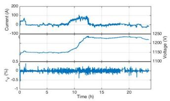
Figure 5. **Top:** BESS current profile simulated through the detailed electrochemical model. **Middle:** BESS simulated voltage profile. **Bottom:** One-stepahead prediction error of the voltage predicted through the SPM.
