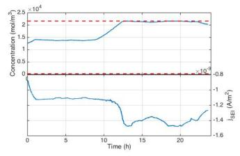
Figure 6. **Top:** Profile of the ion concentration at the anode particle surface (blue line) and its boundaries (red dashed lines). **Bottom:** Profile of the current density of the parasitic reaction leading to SEI formation.
