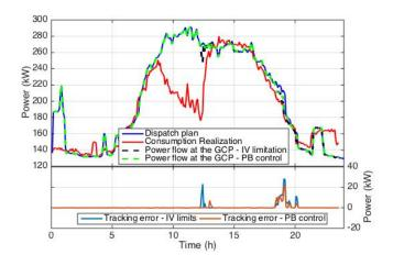
Figure 4. **Top:** 5-minutes resolution profiles of reference power profile, power realization and corrected power profile (both conventional and physics-based MPC). **Bottom:** Tracking error.
