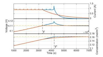
Figure 3. Battery charge with a fixed power set-point. **Top:** cell current, **middle:** cell voltage, **bottom:** anode surface ion concentration. Red lines refer to an MPC based on I-V limits, blue lines refer to a physics-based MPC. Yellow dashed lines in the middle and bottom plots represent the tresholds for the voltage and anode concentration respectively.
