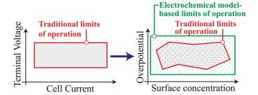
Figure 1. Qualitative comparison of the traditional operational constraints for a Li-ion cell, based on measurable quantities (left) and allowed by the knowledge of actual cell physical states (right) [4].
