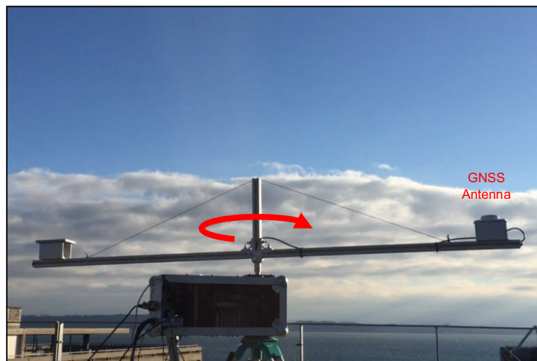
Figure 4 – Rotating arm supporting the GNSS antenna for a circular trajectory. Scenario 1: Neuchâtel's Microcity rooftop. 46^{\circ} 59' 51.3276'' N, 6^{\circ} 56' 44.916'' E; 28-Nov-2016 14h49 GMT+1.
