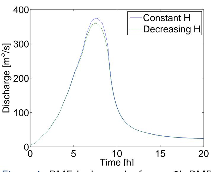
Figure 4: PMF hydrographs from a 9h PMP under constant and decreasing isothermal conditions.
