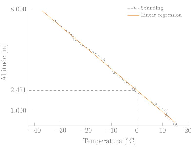
Figure 2: Example of the deduction of the 0°C isothermal altitude H from one mreteorological sounding by linear interpolation.
