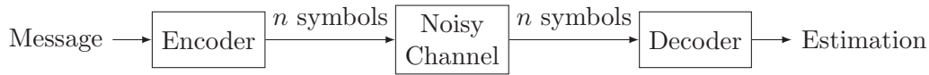
Figure 1.2: To communicate a message, the encoder maps it to n channel input symbols and the decoder estimates the sent message given noisy channel outputs.
