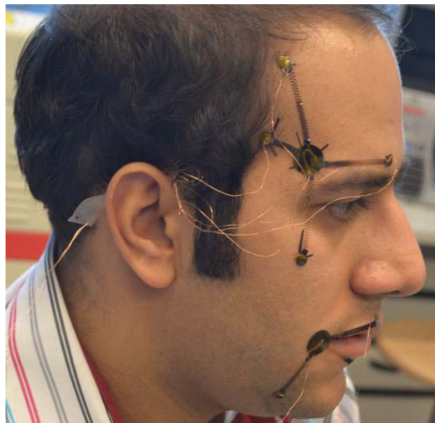
Figure 2.14: A network of stretchable sensors are designed to measure facial movements.
