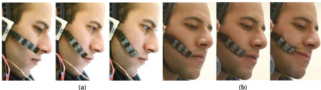
Figure 5.9: Preliminary experiments using a single robogami finger. (a) Performing the initial reconfiguration. (b) Soft actuation on the face.
