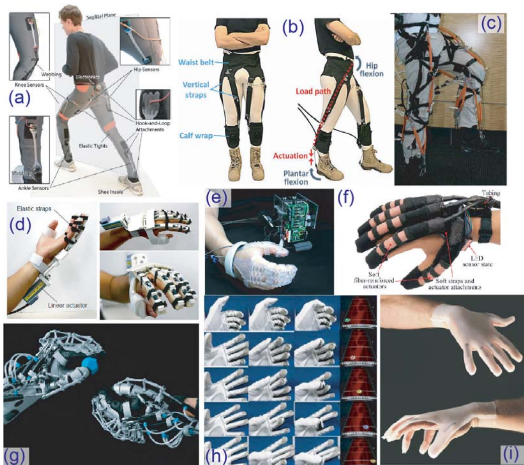
Figure 2: Examples of assistive robots utilizing novel methods of manufacturing, sensing, or actuation. (a) Soft sensing elements for measuring lower body movements [7]. (b) Soft tendon actuation in an assistive device [8]. (c) Soft exoskeleton powered by pneumatic actuators [9]. (d) Hand exoskeleton for rehabilitation, driven by a three-layered sliding spring mechanism [10]. (e) Tendon driven hand exoskeleton that uses novel fabrication methods for fast and cheap customized manufacturing [11]. (f) Hand exoskeleton powered by soft pneumatic actuators [12]. (g) Pneumatically actuated exoskeleton [13]. (h) Music glove uses sensory data to assess the performance of patients [14]. (i) Soft sensing elements embedded in a silicone glove. [15]
