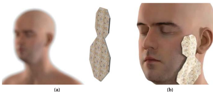
Figure 3: Robogami, a low profile platform with multiple DoFs for developing wearable devices. (a) Different functional layers are embedded in the thin structure of the robot. (b) The robot can reconfigure to the face's shape and perform different tasks, depending on the embedded components.
