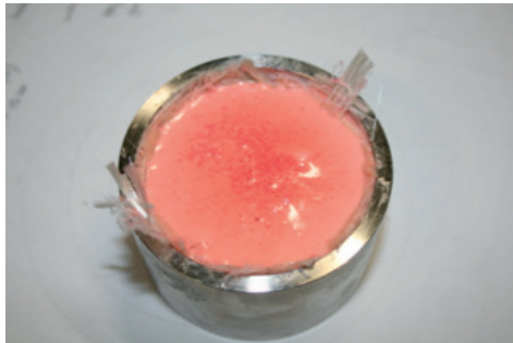
c) Composite structure cured at 60 °C for 60 min.
