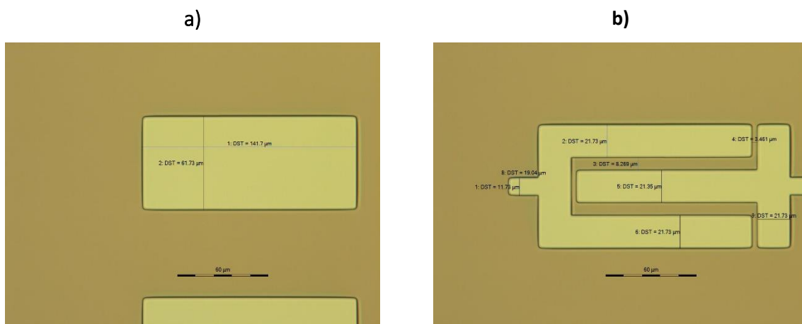
Figure 8 – After the resist development: (a) A plate of exposure dimensions of 60 \times 140 \mu\text{m}^2 with a lift off correction of around 1.7 \mu\text{m} ; (b) Exposure mask settings of the interdigitated electrode: Electrodes width: 20 \mu\text{m} , Anchor length: 18 \mu\text{m} , Anchor width: 10 \mu\text{m} , bus width: 20 \mu\text{m} . The lift off correction is around 1.7 \mu\text{m} .
