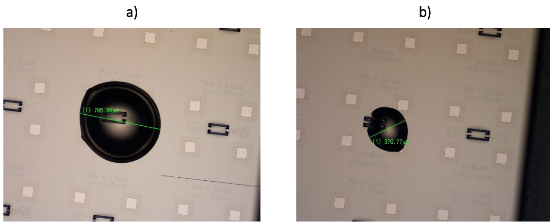
Figure 14 - Droplet deposition on Andrea's design: (a) The droplet has a bigger size (789 \mu\text{m} ) than the whole design (resonator + pads). (b) The droplet can fit in the design without touching the electrodes but the droplet is not accurately deposited and aligned
