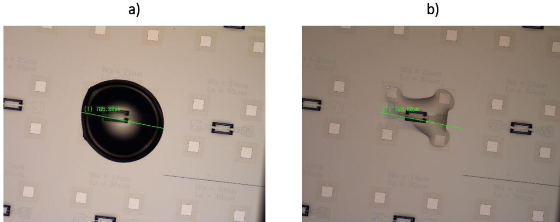
Figure 16 - Liquid is sucked on the pads: (a) Droplet of the size 789 \mu\text{m} deposited on the device. (b) After 1 minute the droplet evaporate and stay on the electrodes
