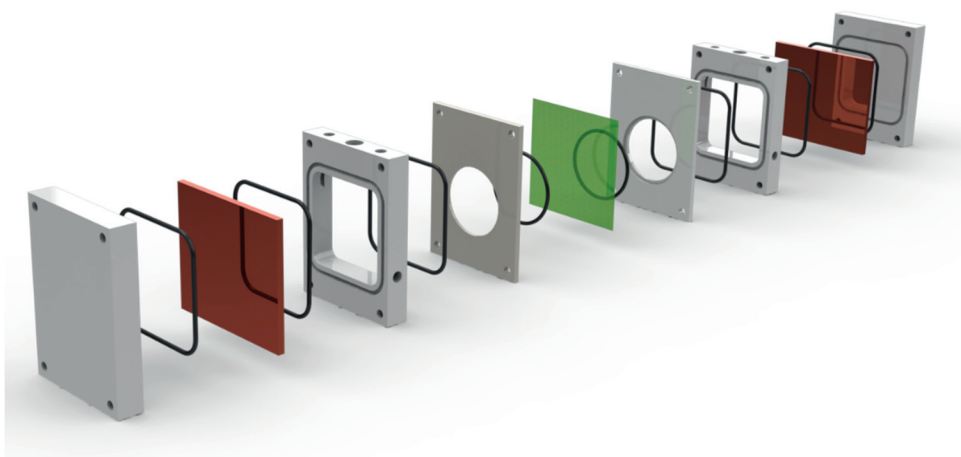
Figure 1-19: CAD Drawing of large scale cell. The copper plates represent the electrodes, whereas the green sheet represents the membrane.
