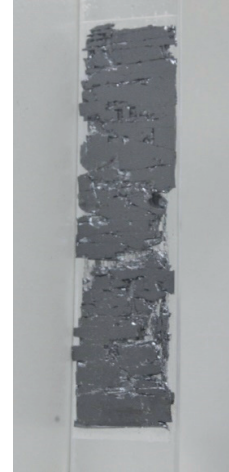
Figure III.1.2: Demolding of Si mold was challenging, as illustrated by the Si mold on a PC preform.
