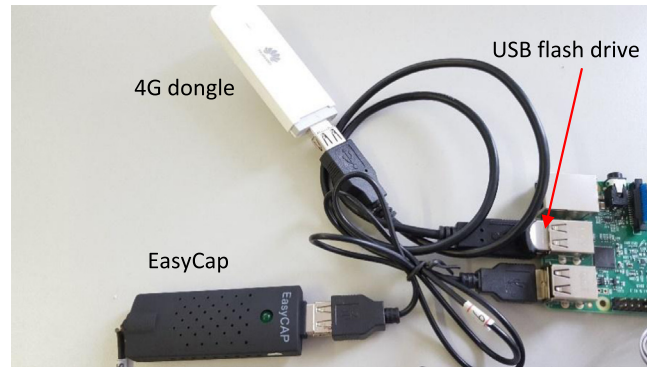
Fig. 5. Connection of different USB devices: 4G dongle, USB flash drive and EasyCAP (converts composite video to USB-compatible format).
