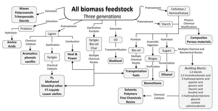
Figure 2.3 The principal conversion routes and products found in an integrated biorefinery.
