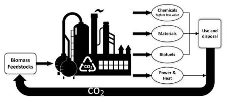
Figure 2.2 A schematic representation of the biorefinery concept with integrated  $CO_2$  use and recycling.
