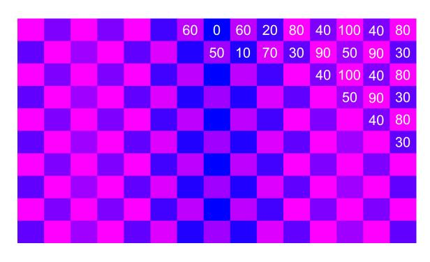
The projected pattern is specifically designed to allow for simultaneous geometric and radiometric calibration of the projector. The red pixel intensities (in %) of the squares vary across the chart. Example intensities are shown in the top-right corner. The printed pattern is composed of a conventional yellow-white checkerboard of identical dimensions to that projected. With this choice of colorants, we are able to isolate the two patterns in different color channels in the captured images.
