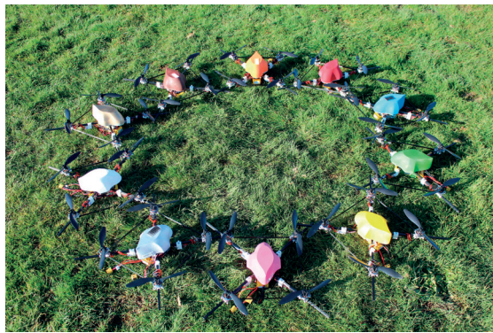
(a) Swarm of 10 hovering platforms used in the experiments
