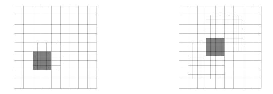
Figure 2: Some examples of two-level meshes for cubic splines (p = 3) of maximum smoothness. In both cases, the highlighted B-splines of level 1 have support included in  $\Omega_1$ , but they are not children of any deactivated B-spline of level 0.
