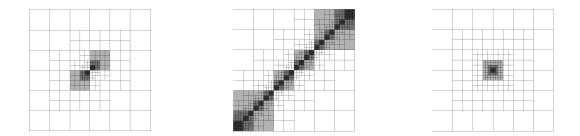
Figure 1: Some examples of four-level meshes for splines of maximum smoothness; we consider quadratics (p = 2) on the left and in the middle, and cubics (p = 3) on the right. In all cases, the meshes are not strictly admissible but they satisfy (28). The domains  $\omega_1$ ,  $\omega_2$  and  $\omega_3$  are highlighted in grey from the lightest to the darkest.
