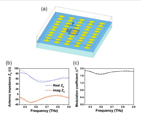
**Figure 3. MS array simulations.** (a) Full geometry domain for the electromagnetic simulation of an array of  $5 \times 5$  MS ( $L_A = 60 \, \mu m$ ,  $W_A = 80 \, \mu m$ ,  $D = 200 \, \mu m$ ,  $P = 250 \, \mu m$ ), highlighting the MS for which the results are plotted in the following. (b) Antenna input impedance and (c) achieved modulation coefficient from 0.45 THz to 0.9 THz for the MS in the center of the array (solid lines) and an isolated MS with the same dimensions (dashed lines).
