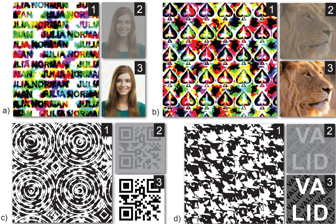
Fig. 9. Sample tempocode frames (1) generated with the different input images and the different dither matrices. The hidden images can be revealed by averaging (2). An inverse contrast reduction operation yields the original input image (3). In all the cases, the target image is recovered by software averaging the original tempocode frames. We have the following parameters (a) for the woman, \alpha = 0.4 , (b) for the lion \alpha = 0.5 , (c) for the QR code \alpha = 0.2 , and (d) for the text, \alpha = 0.3 .
