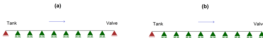
Figure 3.3 – Supporting configurations of the SCP facility with (a) valve anchored and (b) valve released.
