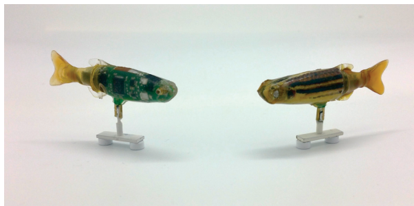
Figure 5.1: The actuated robotic fish lure RiBot, without and with color pattern respectively
