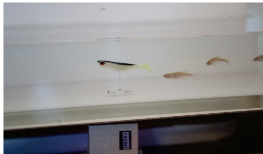
Figure 9.1: The FishBot coupled with a fishing lure that is moving inside an aquarium among zebrafish
