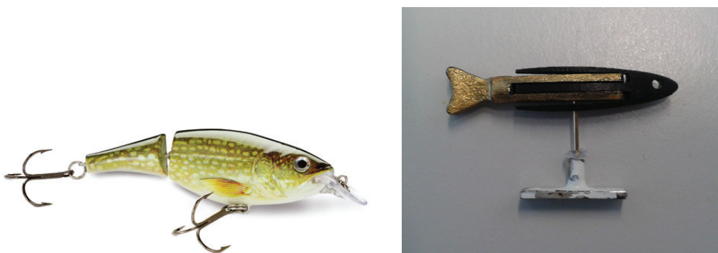
Figure 5.2: Left: Fishing lure X-Rap Jointed Shad actuated passively using the waterflow (Rapala, Finland). Right: Lure with the same size of the zebrafish that was designed to beat its tail when moving with a certain linear speed. The two parts were designed using 3D printing and painted in order to also mimic the color patterns of the zebrafish.
