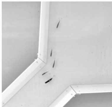
Figure 8.1: Top view of a lure moving inside the two rooms arena among four zebrafish while mimicking the fish locomotion patterns.
