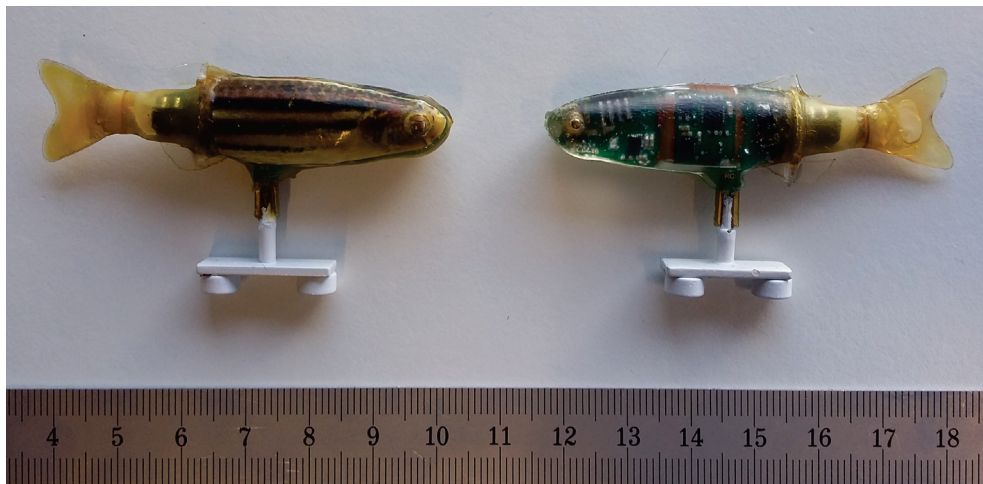
Figure 10.12: Actuated biomimetic lures used in experiment 3. Left: Lure with a zebrafish color pattern. The pattern was printed on the skin of the lure using decals. The pattern was then covered with latex to become waterproof. Right: Lure without any zebrafish color pattern. The PCB with all electronic component that are used for the actuation of the caudal peduncle can be seen from outside.
