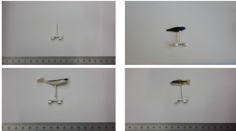
Figure 10.5: The four lures that were tested in Experiment 1. Top Left: the base of the lure composed of an iron plate and a carbon stick of 1.5 mm in diameter painted in white. Top Right: a 3D printed zebrafish replica made of ABS fixed on the base. Bottom Left: a fishing lure mimicking the fish size aspect ratio and beating its tail passively during the motion of the lure underwater. Bottom Right: a lure mimicking the visual appearance and length of a zebrafish, with an increased eye size.
