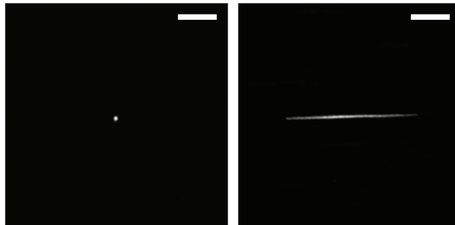
Figure 6.18: Pattern projection through a multicore fiber: line projection (amplitude and phase modulation) . Projection of a DPC focus spot and the line obtained using the same single calibration. Scale bars are 10 \mu\text{m} .
