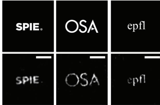
Figure 6.20: Pattern projection through a multicore fiber: complex patterns (amplitude and phase modulation) . Upper row: desired patterns. Lower row: projected pattern. Scale bars are 20 \mu\text{m} .
