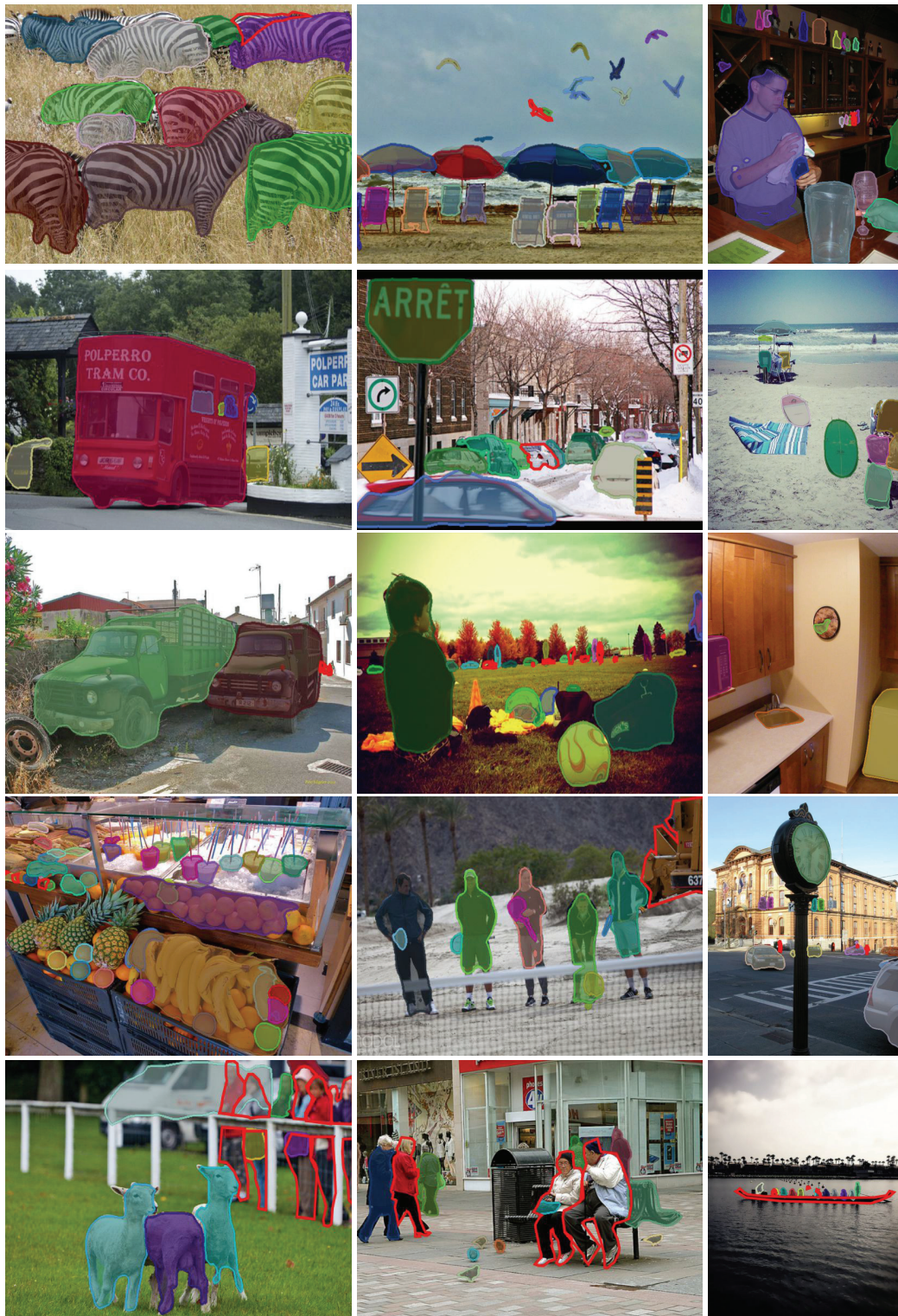
Figure 6.6 – SharpMask proposals with highest IoU to the ground truth on selected COCO images. Missed objects (no matching proposals with \text{IoU} > 0.5 ) are marked in red. The last row shows a number of failure cases.
