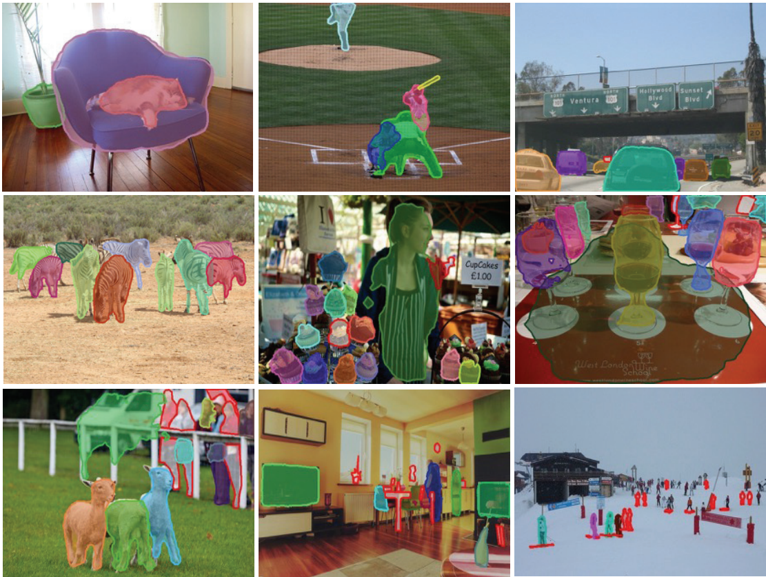
Figure 5.4 – DeepMask proposals with highest IoU to the ground truth on selected images from COCO. Missed objects (no matching proposals with IoU > 0.5) are marked with a red outline.
