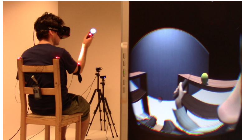
Figure 3.2 – Overview of the system setup. An Oculus DK2 HMD was used as display, and to track head orientation. Optical markers were used for position tracking, while a pair of PSmove controllers were used to track hand orientation and to acquire the target.
