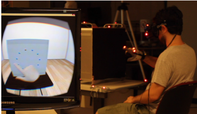
Figure B.3 – Overview of the pointing experiment setup. The subject sit in a chair and wore an HMD and a motion tracking glove.
