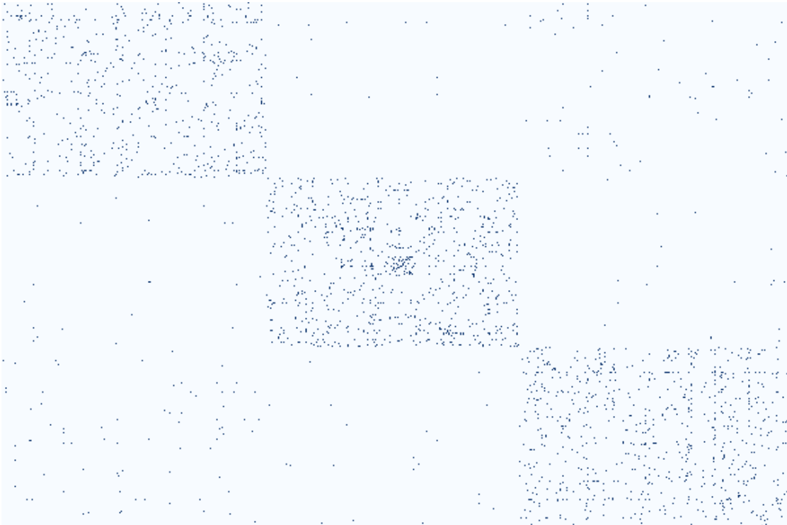
Figure 3.4 – Part of the adjacency matrix of the song graph. The graph is created using the 5 nearest neighbors of each song. Ordered by community ID, the graph is well structured and sparse.
