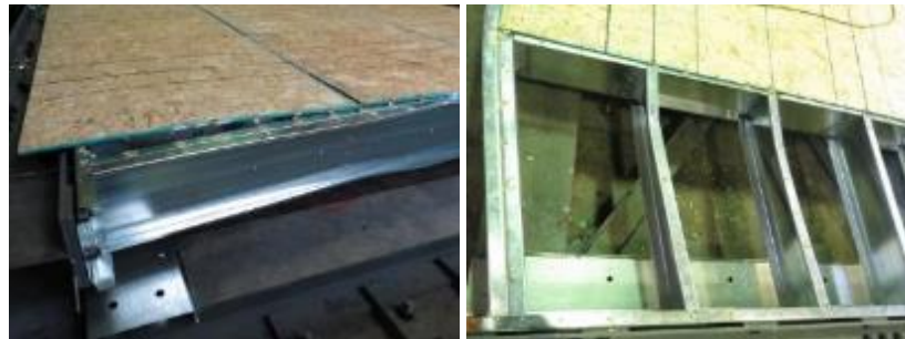
Fig. 9 – Bending action of steel framing, specimen 7-RB-M & 8-RB-C
