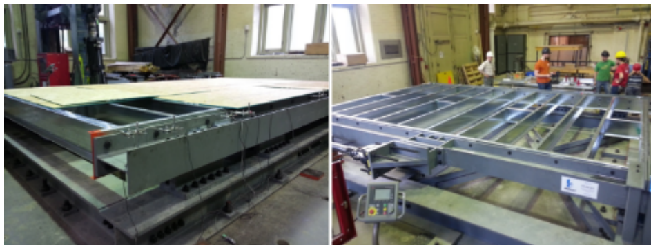
Fig. 3 – Roof specimen (unblocked) attached to test setup
