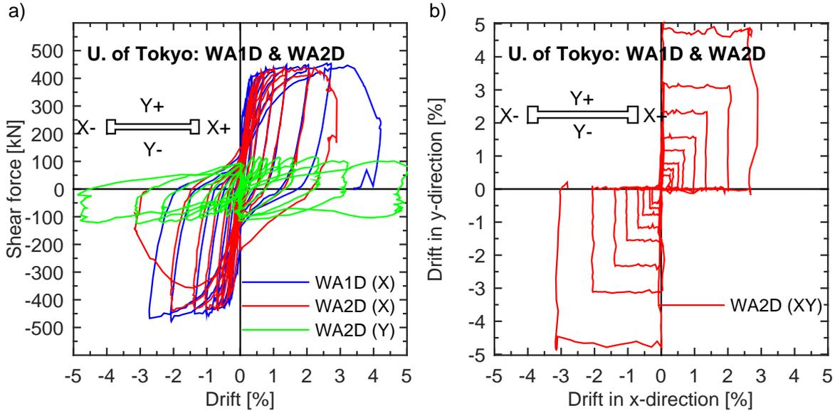
Fig. 1 – Uni- and bi-directional tests on nearly rectangular wall sections of tests from the University of Tokyo (a-b, [9]).
