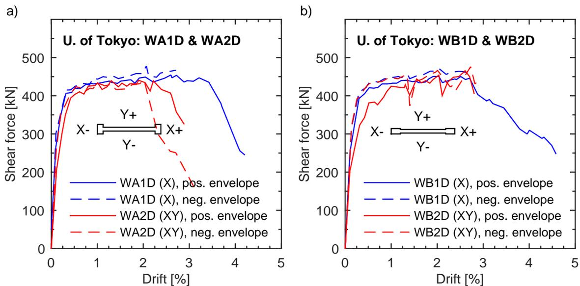
Fig. 2 – Comparison of force-displacement envelopes of uni- and bi-directional tests on rectangular or nearly rectangular wall sections of tests from the University of Tokyo [9].
