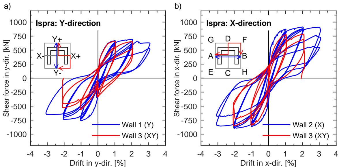
Fig. 3 – Ispra tests on U-shaped walls [12]: Comparison of force-displacement hysteresis for uni-directional loading against force-displacement hysteresis from bi-directional loading (clover leaf pattern): a) Parallel to flanges, b) Parallel to web.
