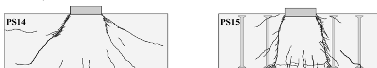
Fig. 3 Schematic representation of saw-cuts of specimens PS14 (left) and PS15 (right) (Simões et al. (2016b)).
