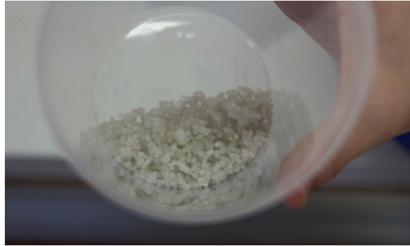
Figure 8.1 PLA2-50 wt% PMMA foam precursors in pellet form containing 0.12 g/g CO 2 .
