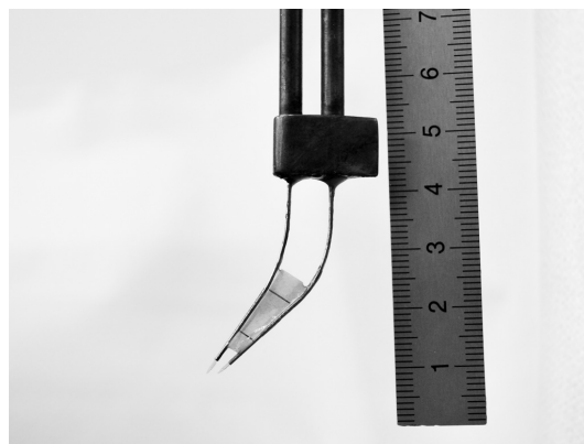
Figure 3.12 – The tips of the fiber optical probe. The optical fibers are protected in thin metallic tubes until the last few millimeters. The sapphire prisms are the light tips at the end of the metallic tubes. The probe is oriented for a flow from left to right. The measuring tape is in centimeters
