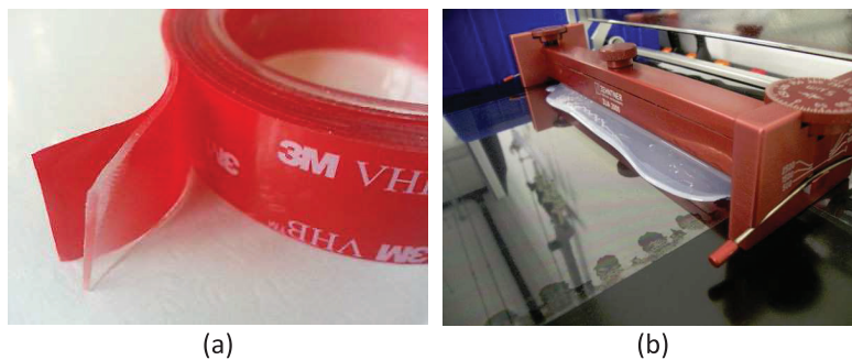
Figure 2.10 – (a)VHB acrylic elastomer commercialized by 3M which comes in 0.5 mm and 1 mm thick films. (b)Two-parts silicone elastomer being formed into a membrane of the desired thickness using a blade-casting applicator. Once formed in to a membrane, the silicone elastomer is heat-cured, and peeled from the casting substrate.
