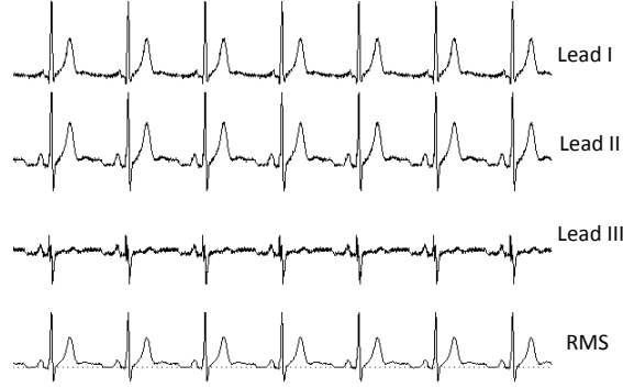
Figure 2.5 – Three-leads acquisition and corresponding RMS-combined signal.
