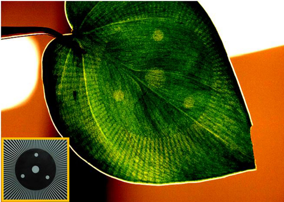
FIG. 7. Philodendron leaf exposed 10 min with a 488 nm laser at 10^3 W/m 2 covered by a transmission mask. Inset shows mask pattern.
