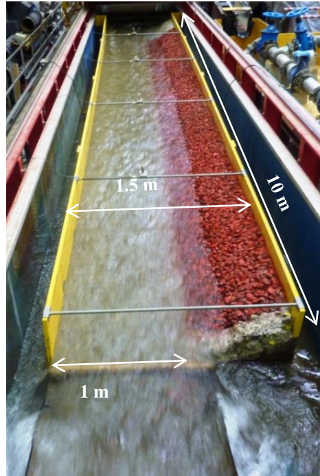
Figure 5.1 Photo of the experimental flume, streamwise view
