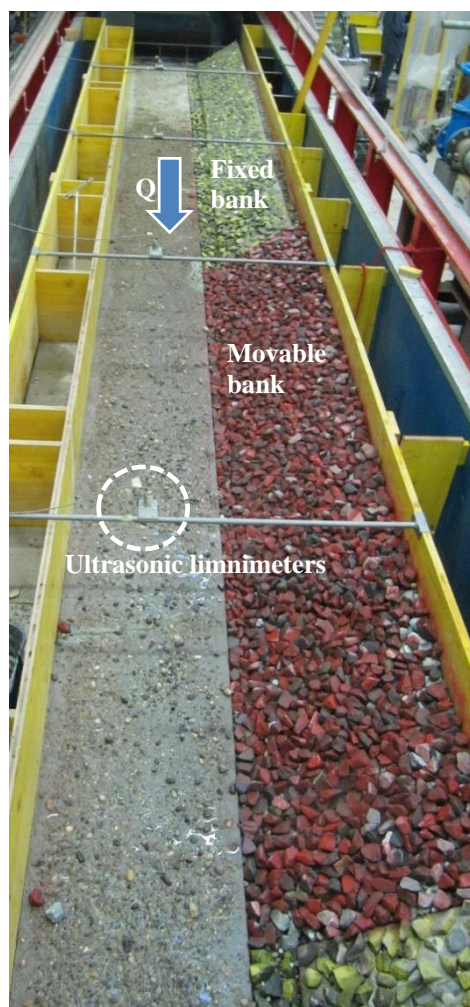
Figure 3.3 View from downstream of the channel presenting the set-up of fixed and movable blocks parts of channel bank and the positions of ultrasonic limnimeter
