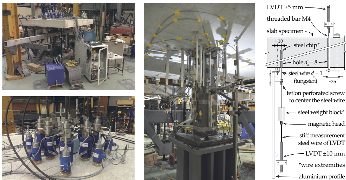
Figure 5.8 Main view of the test specimens ( PB5-6 ) and details of the related measurement devices ( PB4 ) associated to the slab expansion (full and partial thickness variation)
