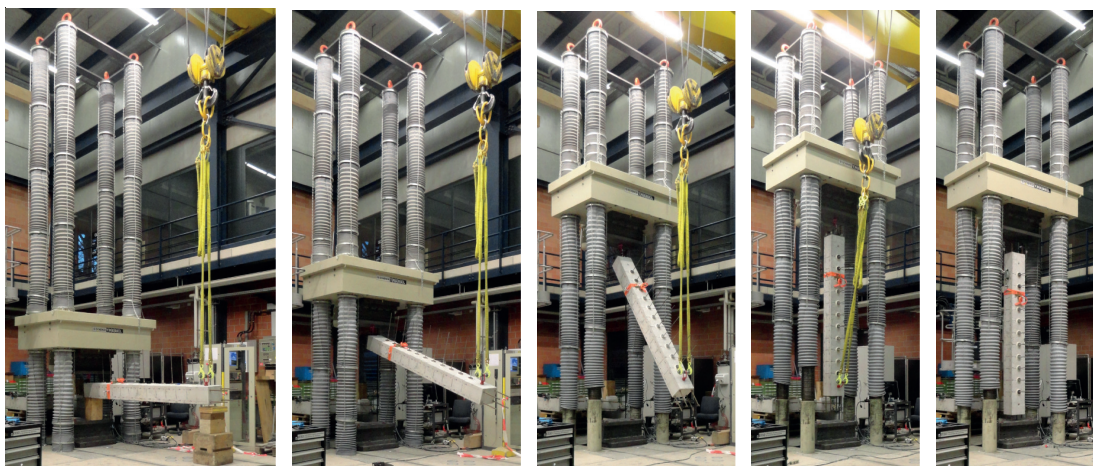
Figure 3.14 Installation steps of the concrete specimen in the test setup prior the crack development and pull-out of the details in the transverse direction
