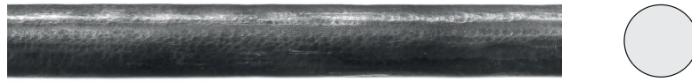
Figure 3.5 Detail of the reinforcement ( d_b = 10 mm) used for the plain hooks (SB16)
